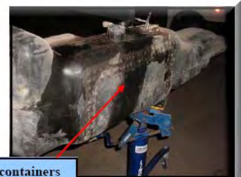
Three metal containers welded and placed inside the fuel tank
