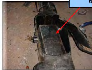
Three metal containers welded and placed inside the fuel tank
