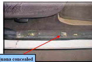
66.68 lbs of marijuana concealed in PVC pipe within rocker panels of vehicle
