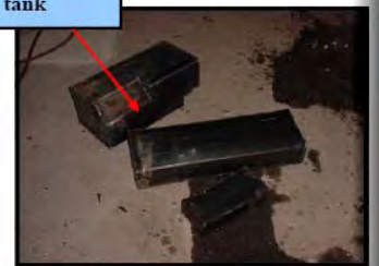
Three metal containers welded and placed inside the fuel tank
